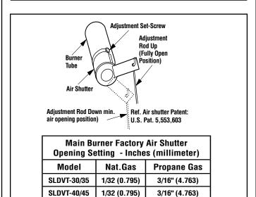
Figure 54 - Burner Air Shutter Adjustment
